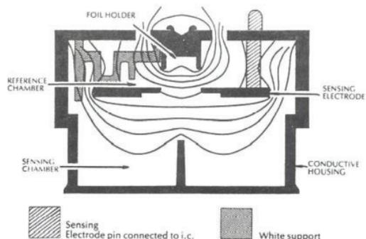
Fig. 2 Diagram showing lines of equipotential for the F900-550 Addressable Ionization Smoke Detector
