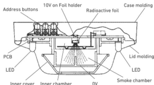
Fig. 1 Sectional View - F900-550 Addressable Ionization Smoke Detector
