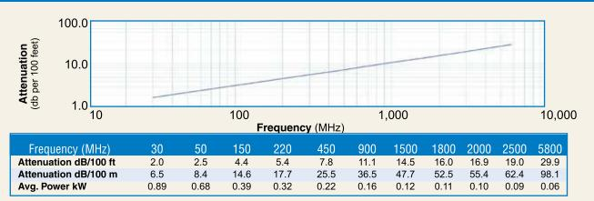
Calculate Attenuation = (0.356859) • FMHz + (0.000470) • FMHz (interactive calculator available at http://www.timesmicrowave.com/cable\_calculators)
